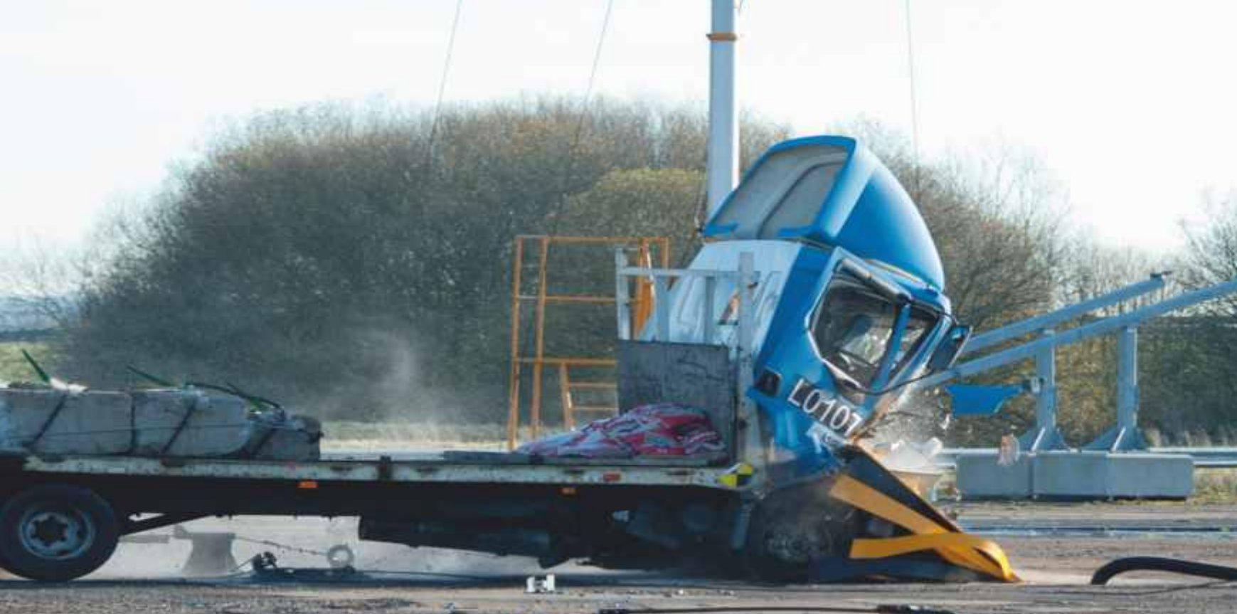
CG10000 Automatic Crash Tested Rising Kerb
