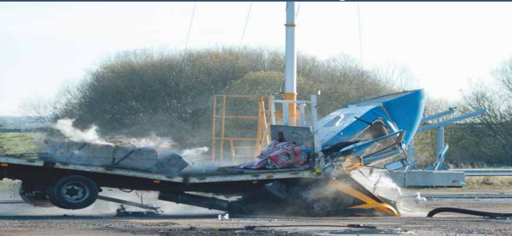
CG10000 Automatic Crash Tested Rising Kerb
